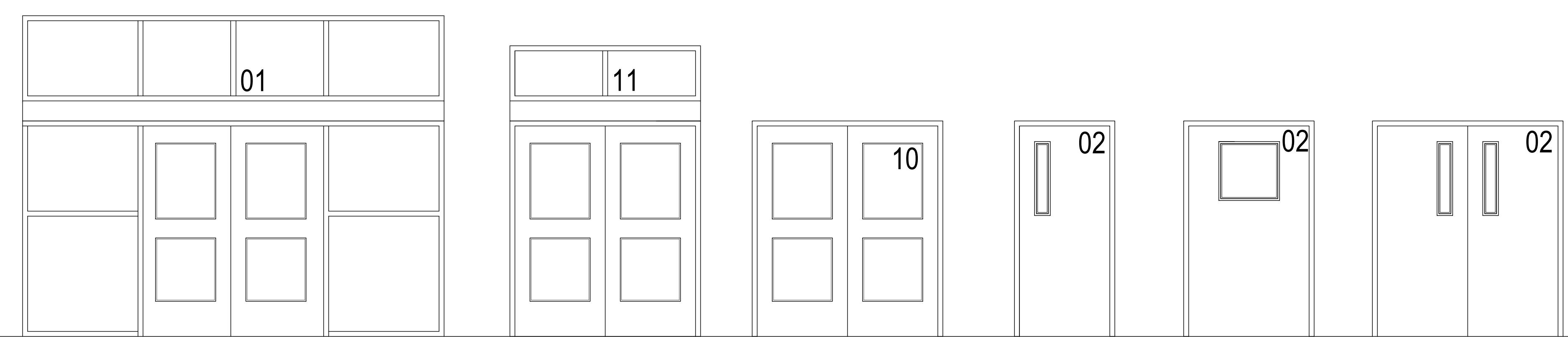
01 DOOR NUMBER LOCATIONS ALL LETTERS ARE SHALL BE 9" TALL VINYL WITH REFLECTIVE FINISH.
